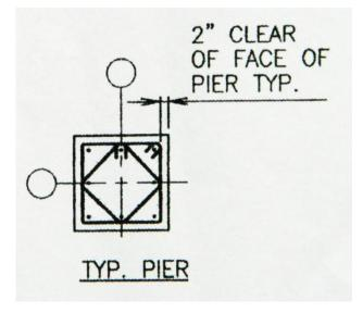
Figure 4: Typical Pier Detail
