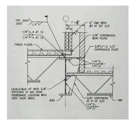
Figure 8: Joists and beam interaction
