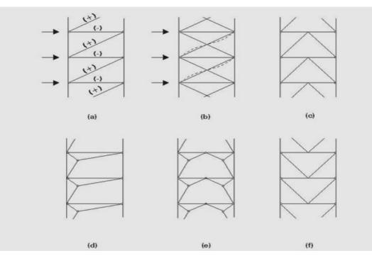
Typical cross bracing and "K" bracing
